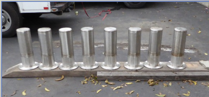
The stainless steel septa screens are an important part of the ion exchange vessel.
