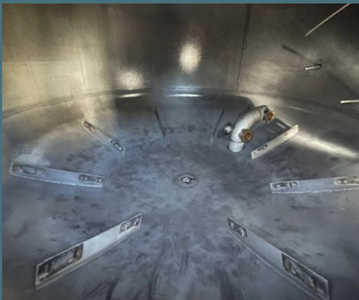
The interior of a GAC vessel after the circular piping system is removed.
