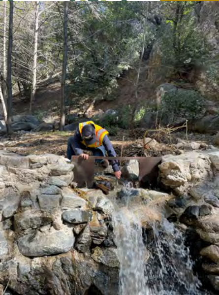
Dave Castillo take a water measurement at one of our canyon weirs.
